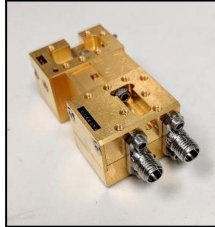
90/120-GHz receiver front end ("WF-RFE")
