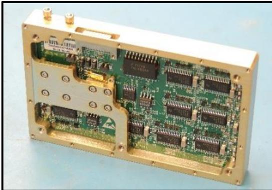
Radiometer back-end processor ("WF-IFP")
