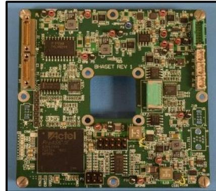
Payload control and data handling board
