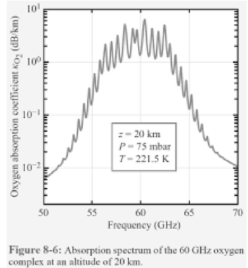
Figure 8-6: Absorption spectrum of the 60 GHz oxygen complex at an altitude of 20 km.
