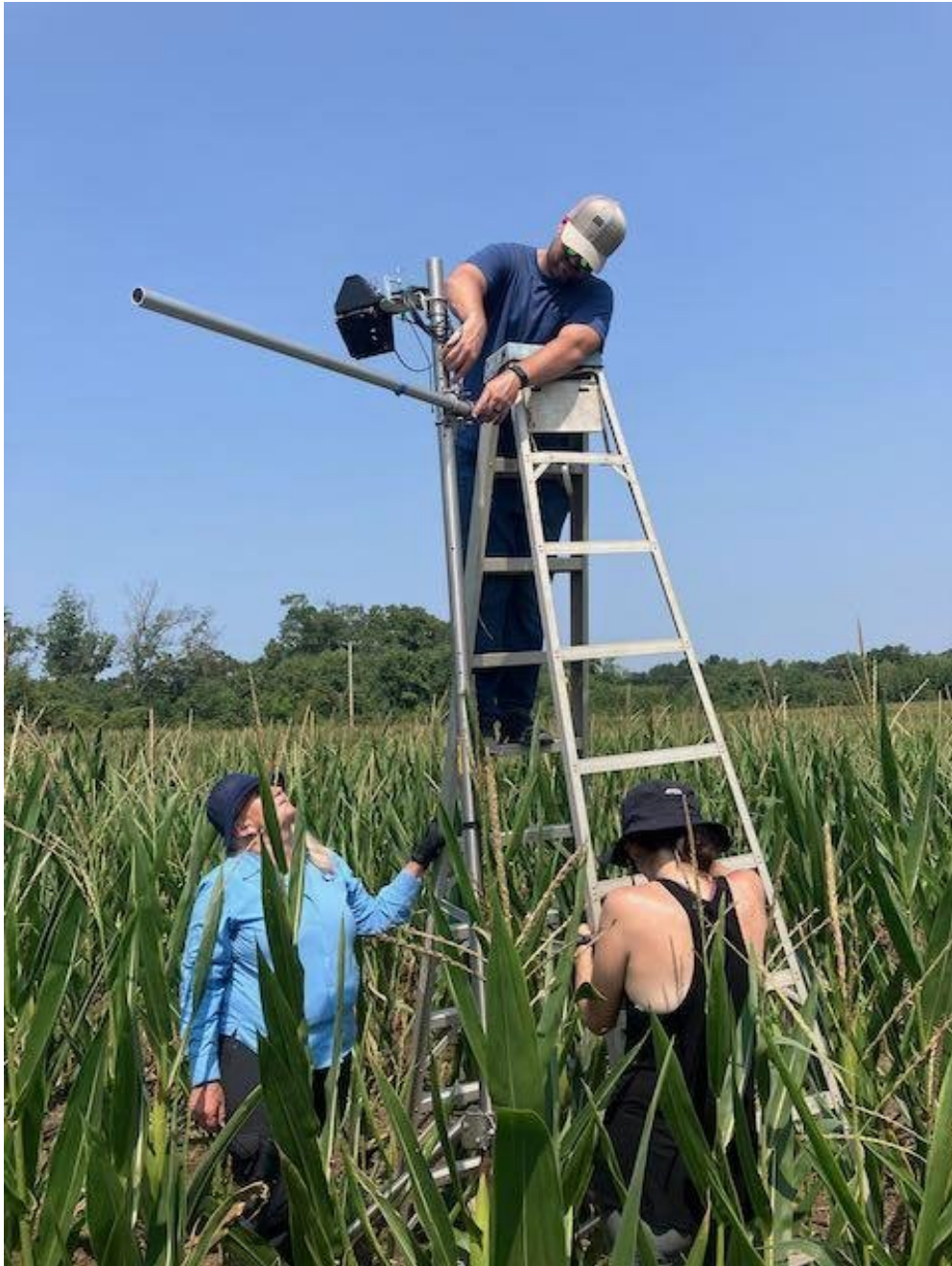
Photo left shows Petya Campbell installing a FLoX (Fluorescence Box) at the USDA cornfield down the road from Goddard, which measures canopy reflectance and solar induced fluorescence. She is working with Maggie Wooten (SSAI) and Will Wagner (SSAI).
