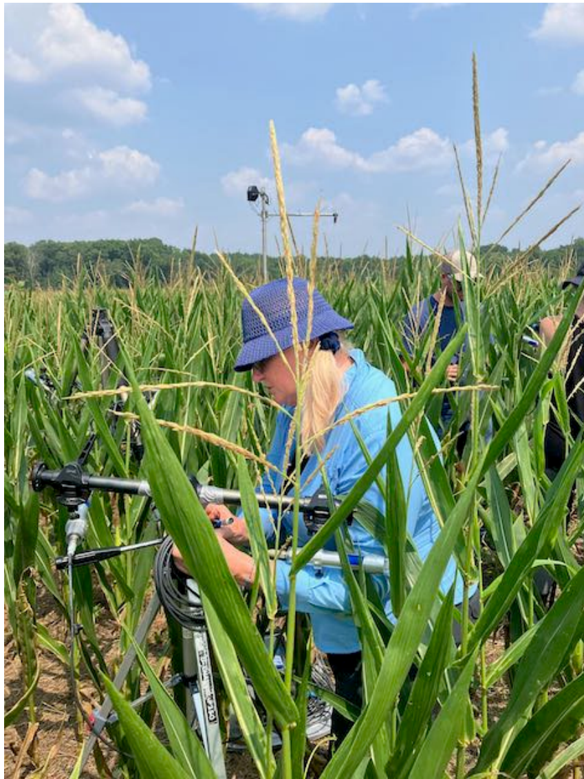
Photo: Petya Campbell installing a MoniPAM in a cornfield in the Beltsville Agricultural Research Center.
