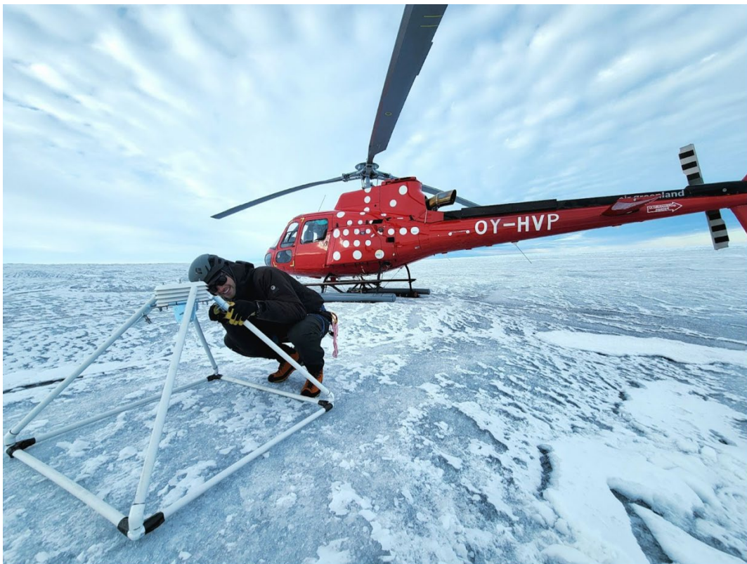
Image: Field work in Sermeq Kujalleq (Kangia), Greenland performing a field installation on the ice sheet with GNSS antenna, receiver box, solar panel, and temperature sensor. Credit: Elizabeth Ultee.
